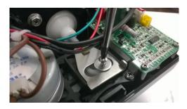
8) Remove Phillips button head screw from centre of gear that is holding piston rod.
