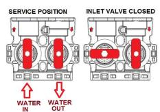
3) Open a faucet anywhere in the house to release the pressure inside the unit. Some water will come out after which the faucet will run dry. Close the faucet & also close the outlet of the bypass valve
