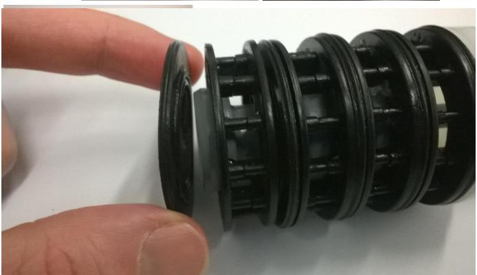
12) Re-assemble the spacers and seals in the same manner they were removed from the valve body. Seal first followed by spacer. The seals and spacers are symmetrical, so the direction they face doesn't matter. After all seals and spacers have been inserted, push the piston rod into the centre.
